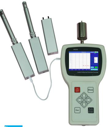
The Handheld Particle Counter **CTZ-PC-H630** is reliable and easy to use. It is handheld, ergonomically designed, and light. **CTZ-PC-H630** simultaneously counts airborne particles in six different size ranges. It has a 480×320 high-resolution colorful LCD screen. The count data is displayed on the screen as the total number of particles (cumulative count). Data can be easily downloaded to a computer or printed with an optional printer.
