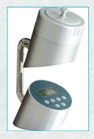
Portable Biological Air Sampler is designed according to the multibeam hole particle effect and isokinetic sampling principle. It more accurately absorbs airborne organisms. While sampling, airborne particles attach to the agar surface of substrate materials through small holes. Organisms in the particles form colonies on top of the agar plate after incubation and these can be counted.
